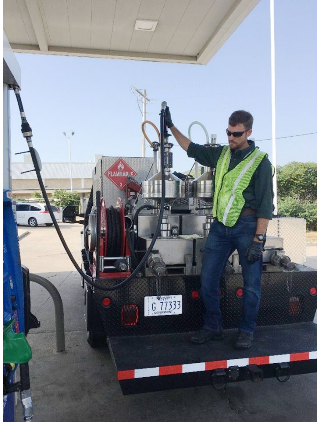
An MDAC Petroleum inspector verifies the accuracy of a gas pump.
