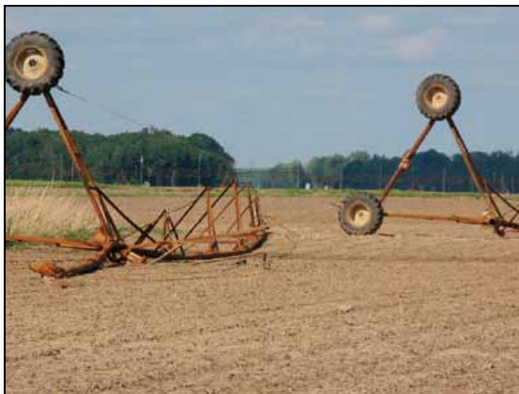
Irrigation equipment could not hold its ground as the April 24 storms turned these center pivots upside down in a corn field near River Road in Yazoo County. (Photo by Phillip Vandever/MSU Extension Service)
