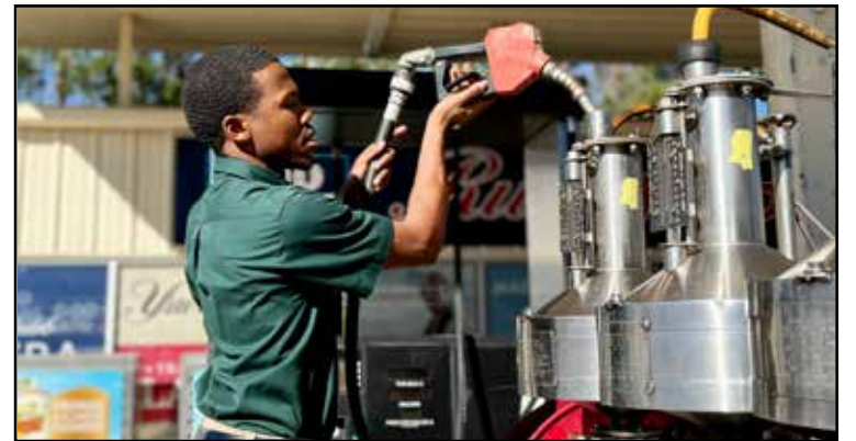
MDAC's Petroleum Inspector, Jamarcus Davis, checks the accuracy of the pumps at a local gas station with his slide-in calibration unit to ensure that the consumer is getting the quantity of gas that they pay for.
