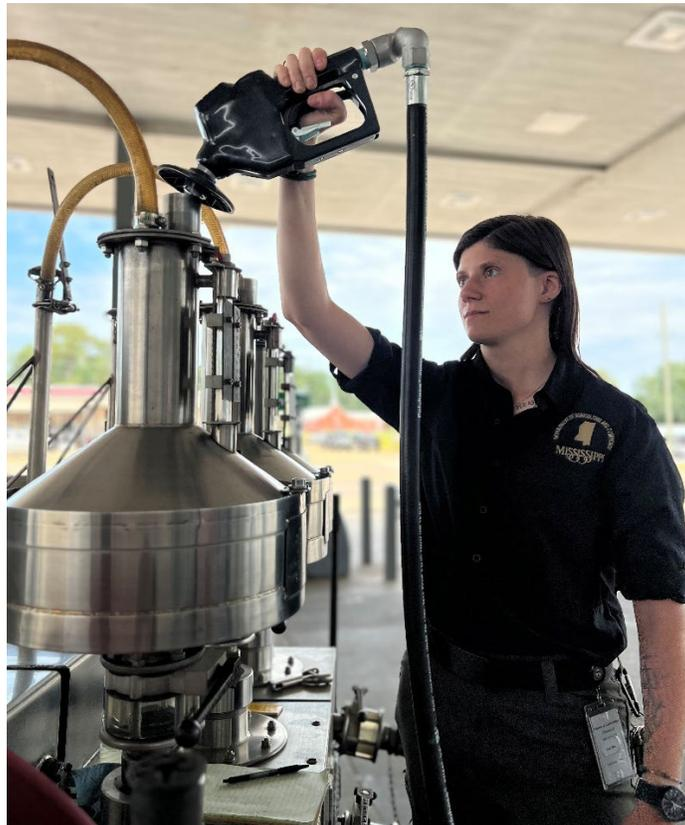
**A MDAC Petroleum inspector verifies the accuracy of a gas pump.**
