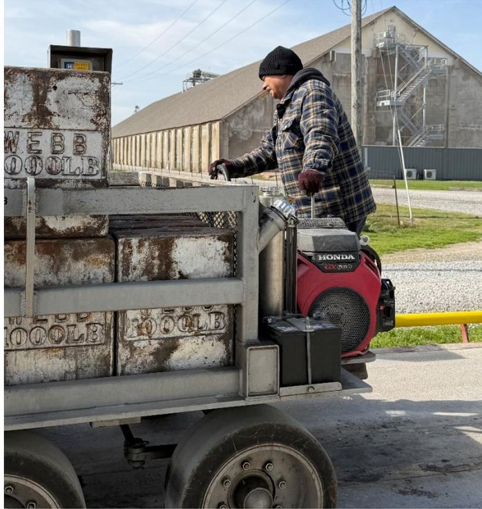
**A MDAC Weights and Measures inspector testing a vehicle scale for accuracy.**
