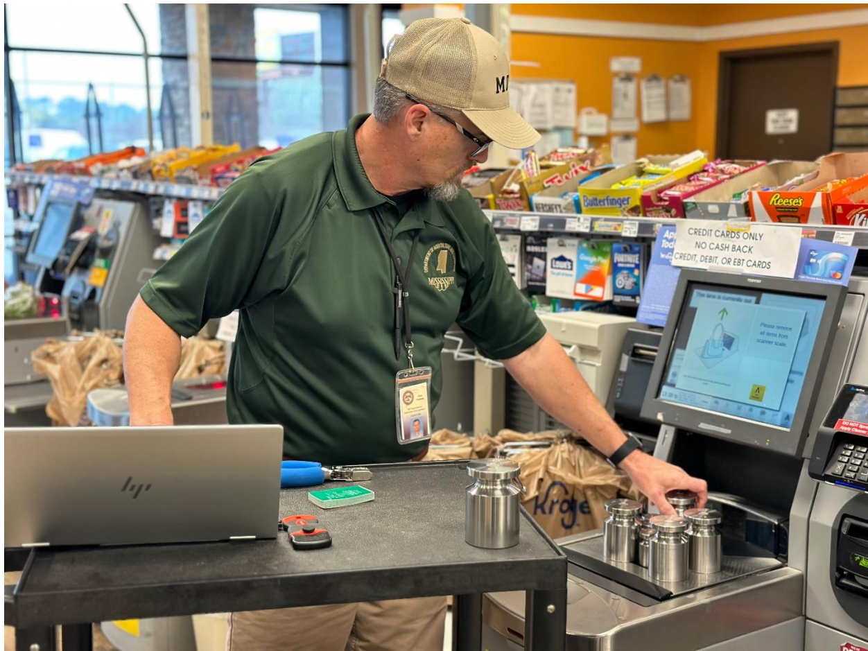
An MDAC Consumer Protection inspector checking a grocery scale for accuracy.
