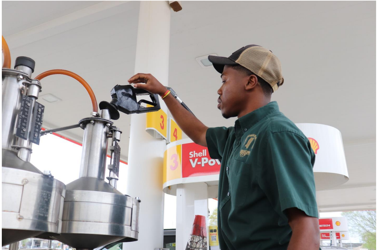
An MDAC Petroleum inspector verifies the accuracy of a gas pump.
